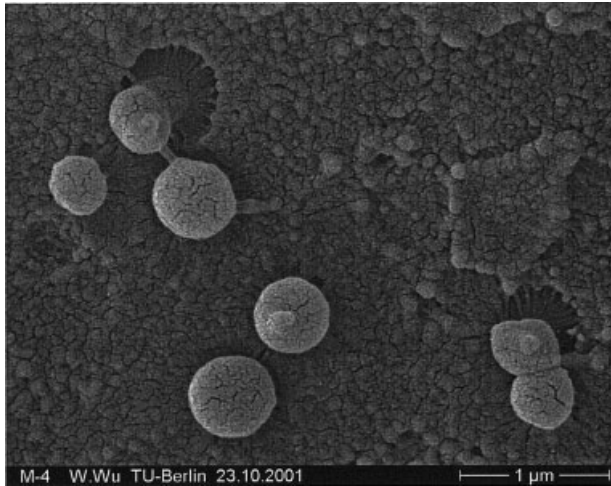
Figure 7 SEM photograph of the fracture surface of an extruded sample of a PET/PEN blend (80/20).
