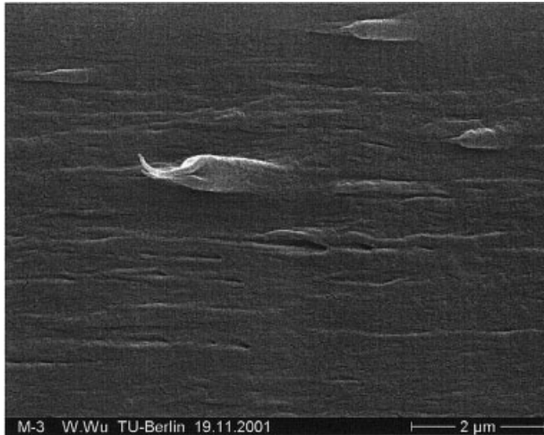
Figure 11 SEM photograph of the tearing fracture surface of a biaxially oriented film of a PET/PEN blend (90/10).
