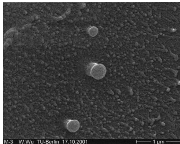
Figure 6 SEM photograph of the fracture surface of an extruded sample of a PET/PEN blend (90/10).
